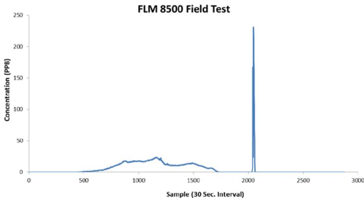
US EPA conducted field testing results. 30 second exposure to high concentration Isobutylene.
